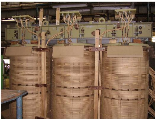
Fig. 3 (a) : 100 MVA power transformer without any deformation
