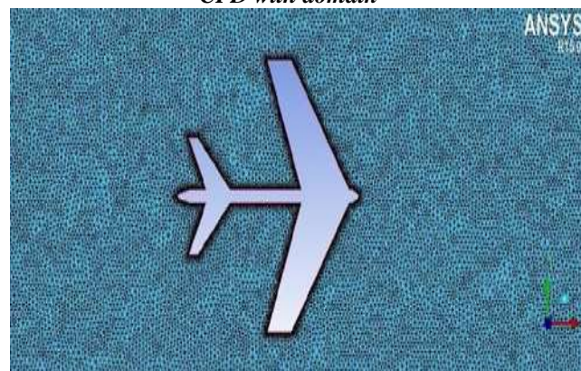
Fig. 10 2D model of FSW aircraft with FSC with meshing in ICEM CFD with domain
