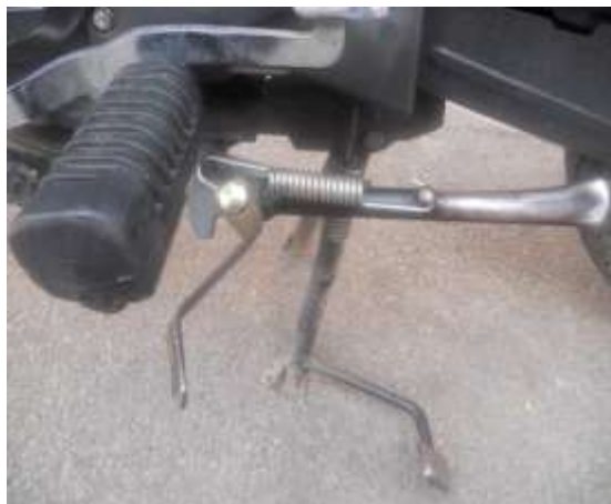
Fig. 3 Released position of the side stand with assembled side stand lock link
