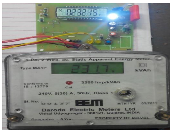
Fig. 15 Comparison between Energy meter and Smart meter
