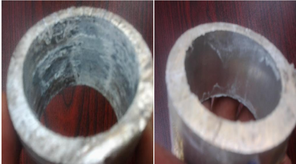
Fig. 4.9: Coated sample after corrosion test during 24 Hrs Fig. 4.10: Base metal after corrosion test during 24 Hrs
