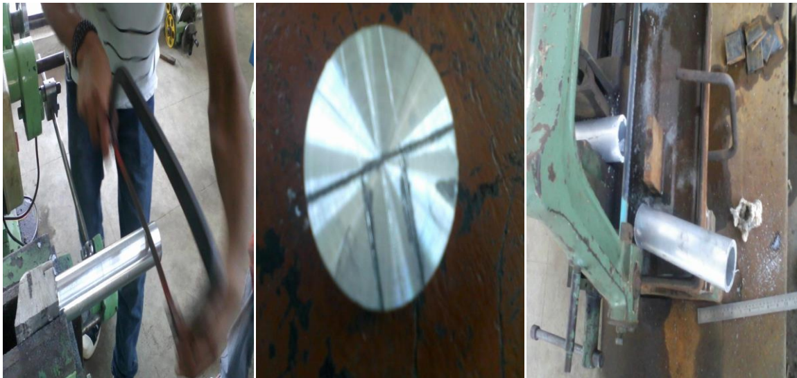
Fig. 3.4: Preparation of tool from cylindrical rod Fig. 3.5: Pipe material is cut into required size
