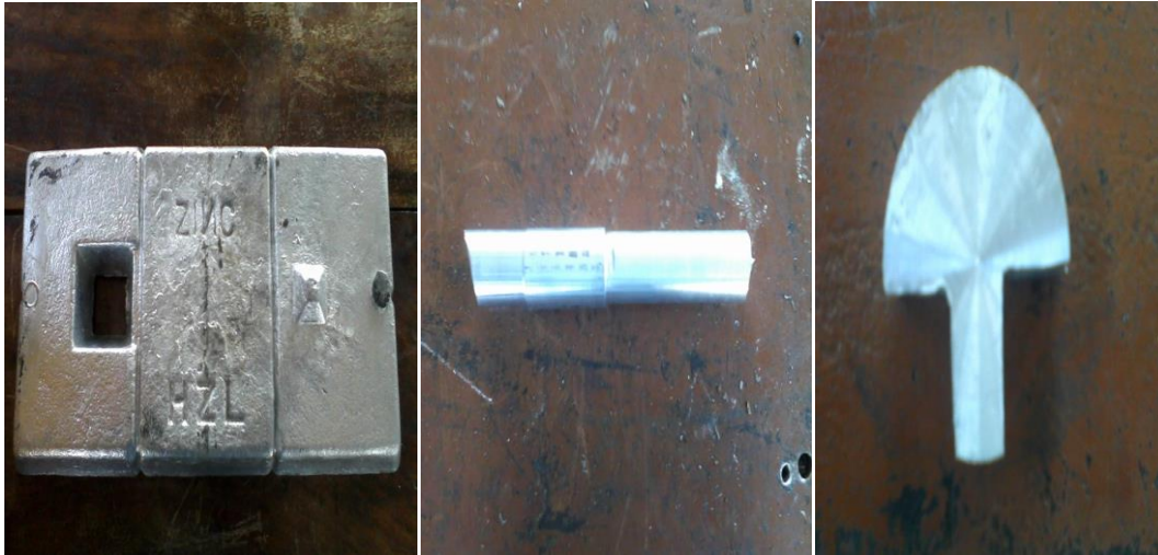
Fig. 3.1: Zinc billet Fig. 3.2: Zinc cylindrical rod Fig. 3.3: Zinc tool material
