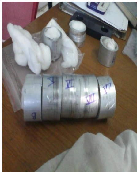
Fig. 3.7: Sample prepared for corrosion test Fig. 3.8: Corrosion testing machine
