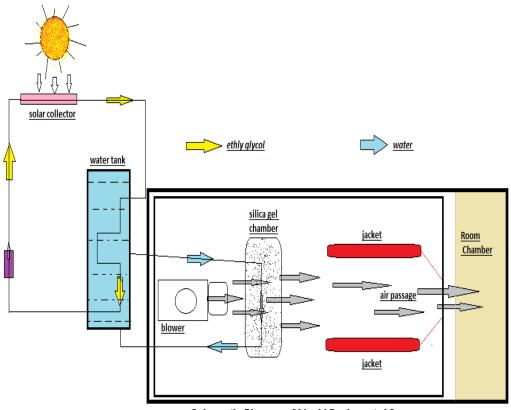
Schematic Diagram of Liquid Desiccant AC
