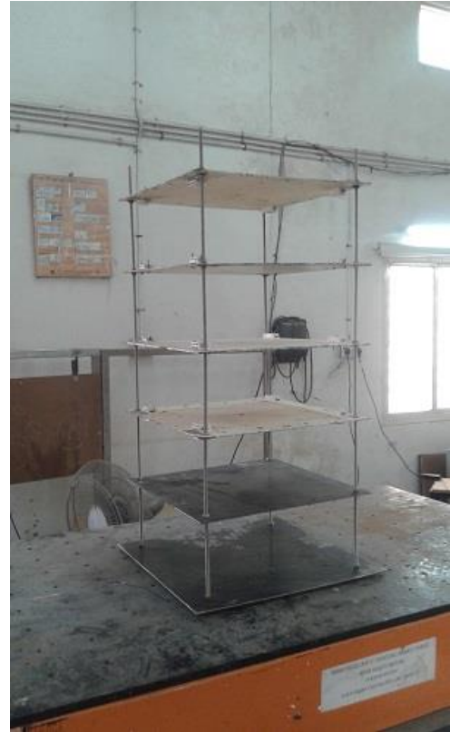
Figure 2. Final setup of the shaking table tests for the structure with Fixed base condition
