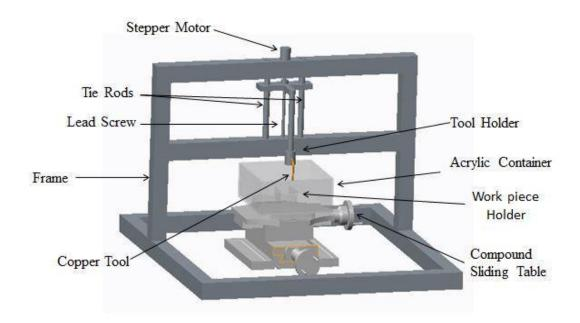
Figure 2.1 Creo model of ECM setup
