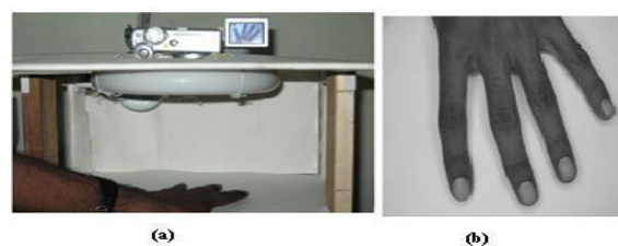
Figure 2 (a) acquisition of finger back image (b) acquired image
