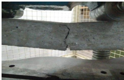
Figure: 5 Failure Pattern Observed In Beam
