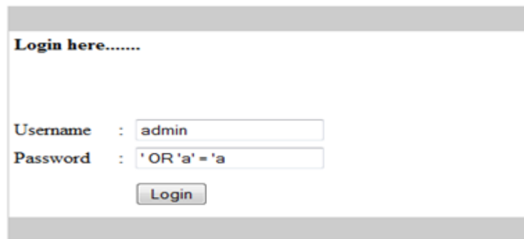
Figure 2: Insert data for Authorization Bypass using SQL command Injection
