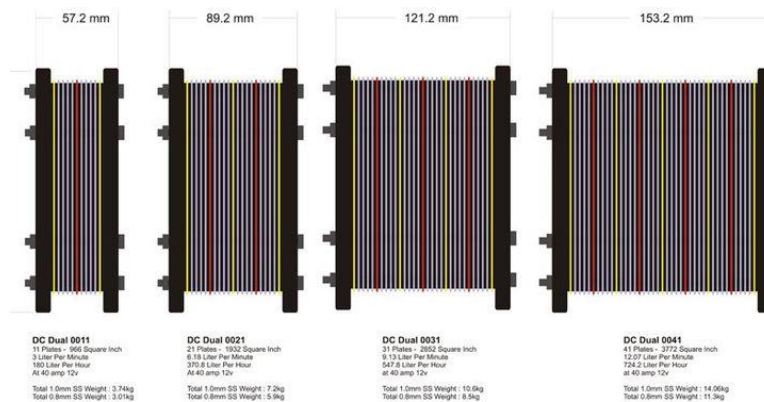
Fig 3: Schematic diagram of HHO Generator
