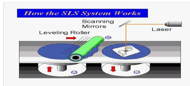
Figure 2 Diagram of Selective Laser Sintering
