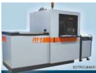
Figure1 SLS Cusing Machine
