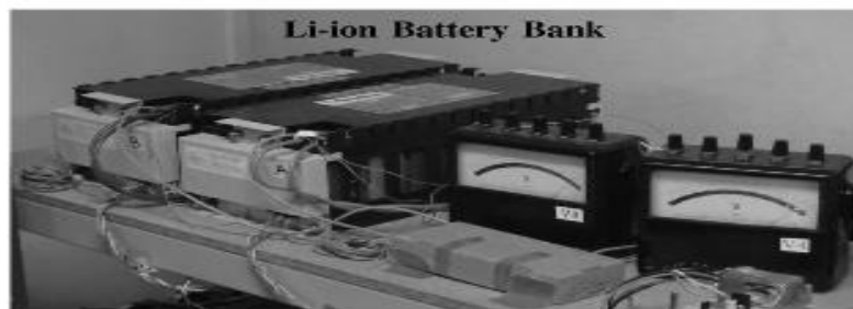
Figure 1.2 Photo of the two Li-ion battery modules used for experiment, each of which is rated at 26.6 V and 40 A·h
