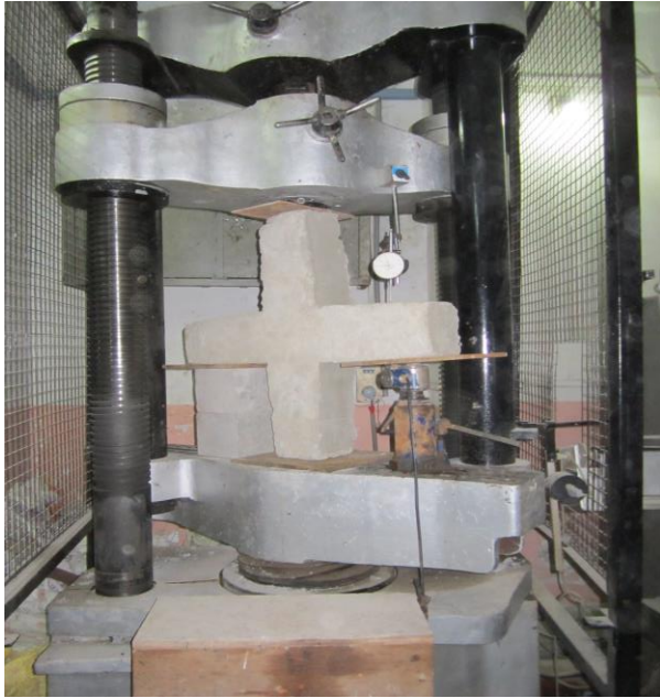
Figure 7. Test arrangement for Virgin Specimen
