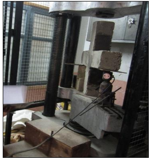
Figure 8. Test arrangement for Rehabilitated Specimen
