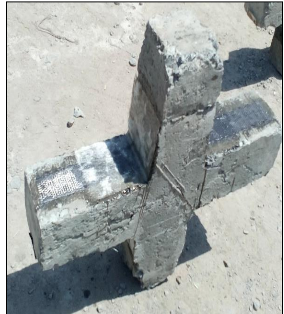
Figure 6. Hybrid Wrapping of CSM on CFRP
