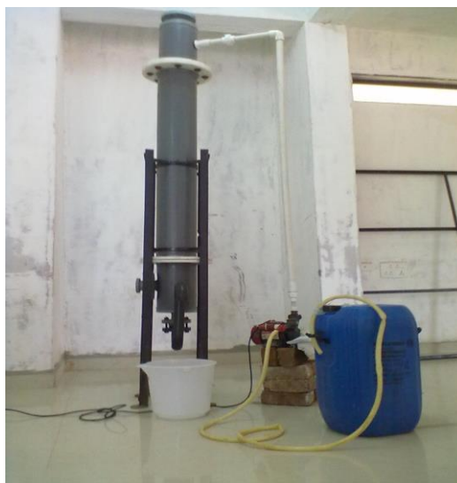
Fig 7: Reduction by Stripping Tower at Pilot scale.
