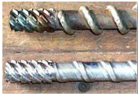
Fig 2: Wear of screw
