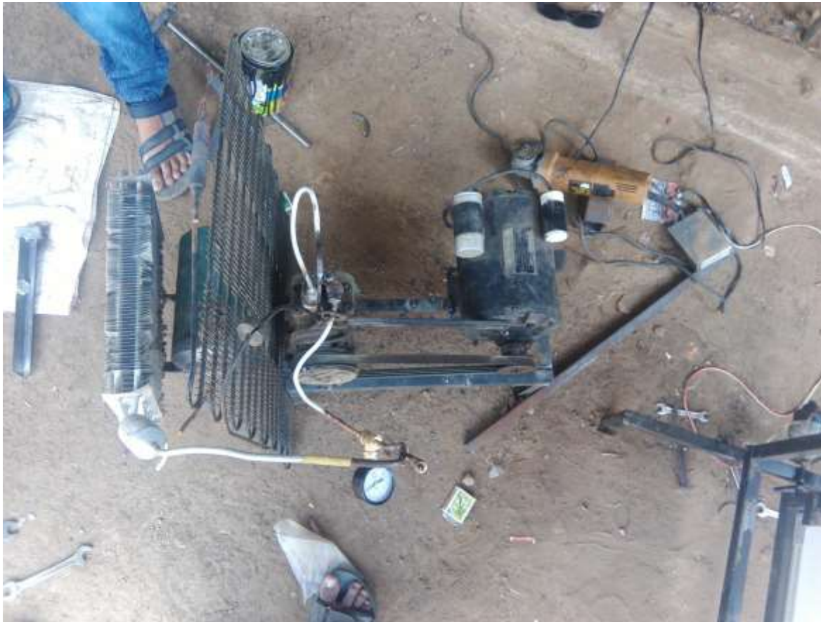
Fig.1 vapour absorption refrigeration system
