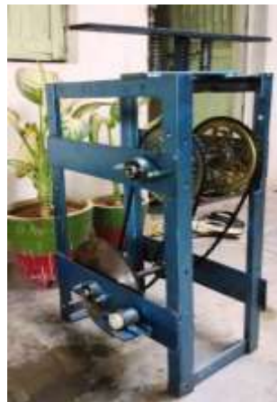
Figure 1. Model of Footstep Power Generation System
