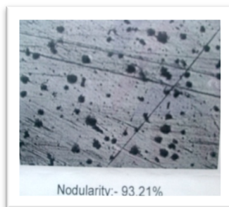
Fig 7:- Microstructure of Gray cast iron having 0.040% Mg, Without Etchant
