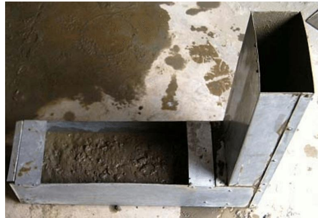
Figure 2 L-Box test Apparatus
