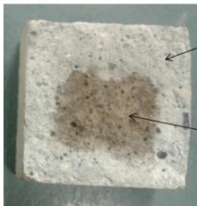
Figure 5 Acid Ponding Test
