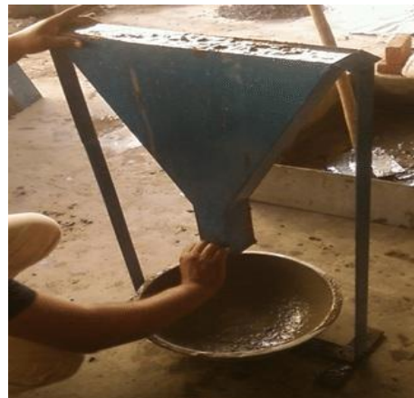
Figure 1 V-Funnel test Apparatus
