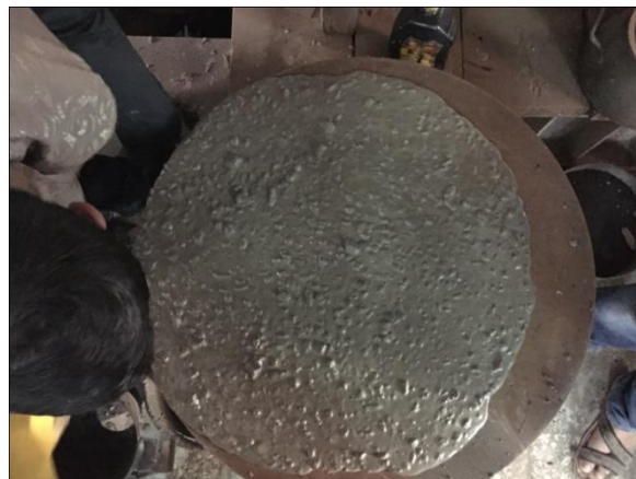
Figure 3 Slump Flow Test
