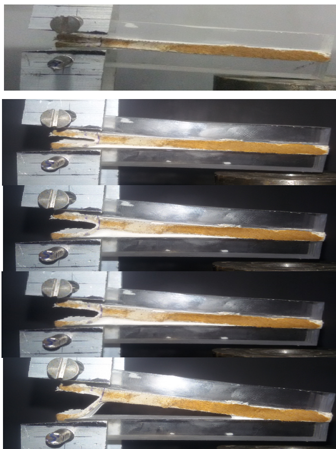
Fig.4.5 Failure Sequence of the specimen
