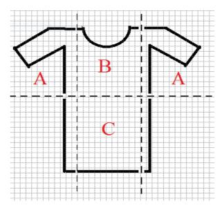
Above diagram shows how the actually cloth is being folded step by step using this machine using only 3 Servo motors. For this project the platform is used is 5mm plywood is used. Servo motor is used are all metal gear and uses all metal horns to grab the wooden platform sections.
