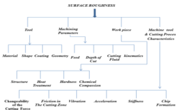
Fig. 1 Parameters affects the surface roughness
