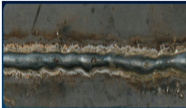
Figure 2.7 Travel Speed Too Fast
