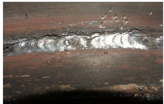
Figure 1.3 (b) Incomplete Penetrations
