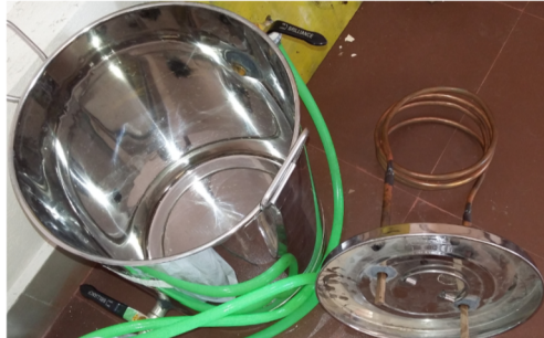
Figure 3. Inner side of the FPC alternate stainless steel tank showing the coil and lid part
