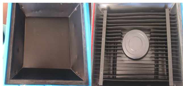
Figure 6. Experimental setup of box type solar cooker using finned absorber plate
