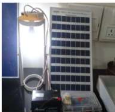
CFL Based lantern pictures during all the operations on open holder design of the solar lantern in minimum height setting
