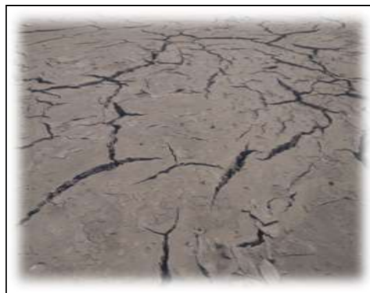
Figure 4: Waste paper sludge in semi dry form
