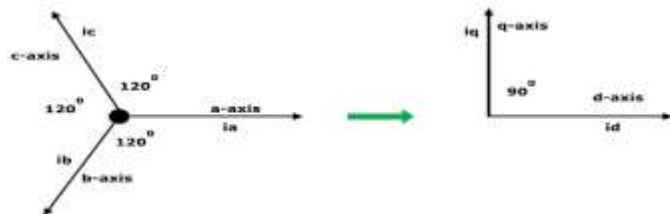
Figure 5. a-b-c to d-q-0 transformation (park transformation)
