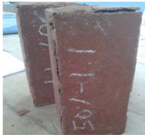
Fig 4: Failure of brick after testing
