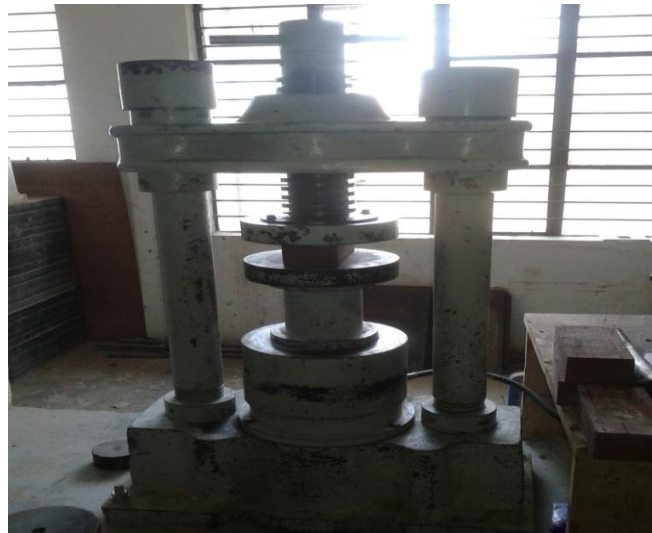
Fig 8: Testing of bricks after immersion in sulphate solution.
