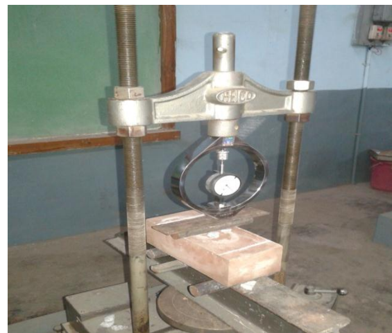
Fig 6: Testing of bricks for flexural strength
