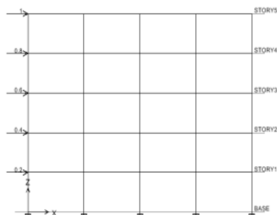
Figure 3: Lateral Loading Pattern
