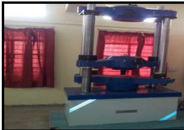
Fig.27 Static Test Set Up For Both Composite And Steel Shock Absorber.
