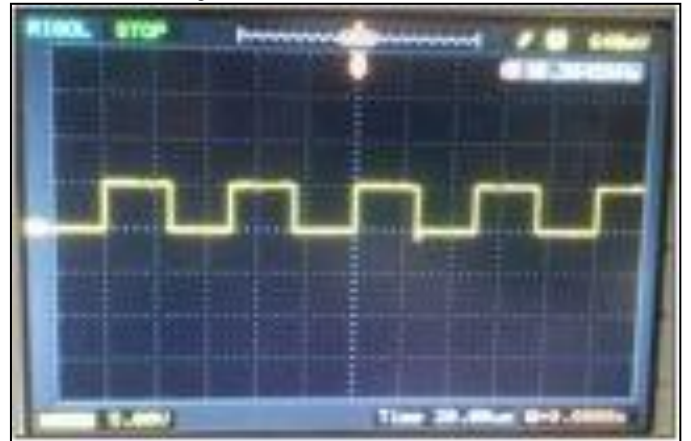
Figure 22: PWM pulse from PIC Microcontroller board.
