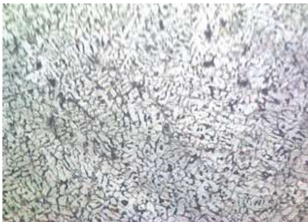
Fig. 16 Optical microstructure of unreinforced A356 alloy with 8 wt. % (SiC + Al 2 O 3 ) particles at 200X
