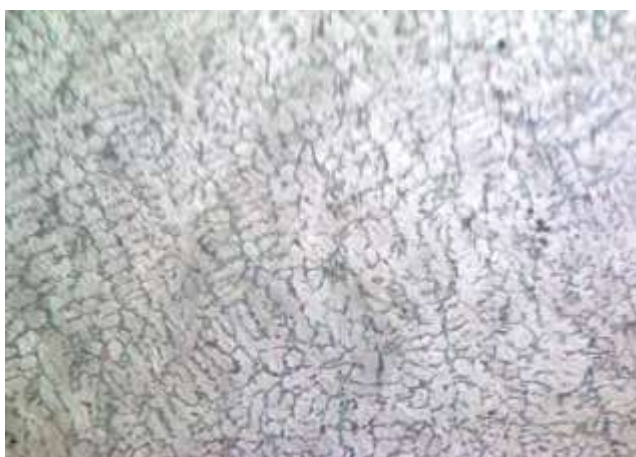
Fig. 17 Optical microstructure of unreinforced A356 alloy with 12 wt. % (SiC + Al 2 O 3 ) particles at 200X
