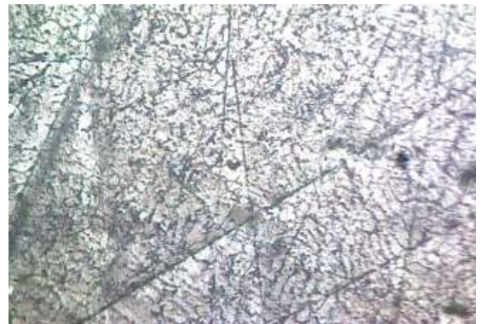
Fig. 13 Optical microstructures of unreinforced A356 alloy with 8 wt. % Al_2O_3 particles at 200X
