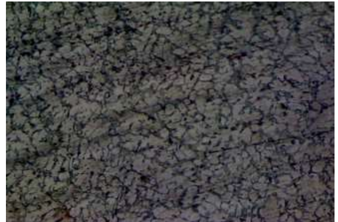
Fig. 12 Optical microstructures of unreinforced A356 alloy with 4 wt. % Al_2O_3 particles at 200X
