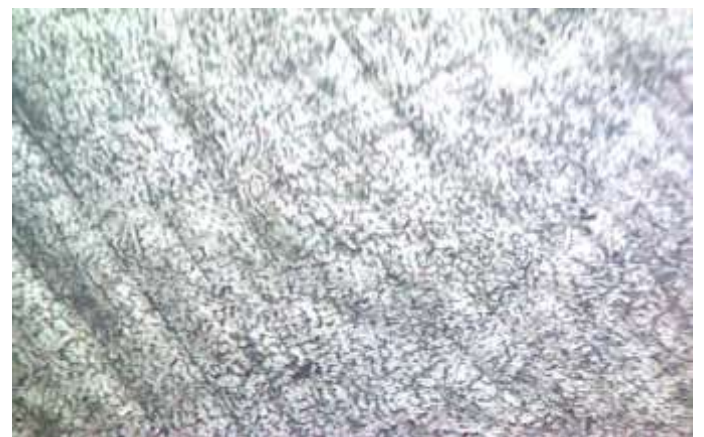
Fig. 14 Optical microstructure of unreinforced A356 alloy with 12 wt. % Al_2O_3 particles at 200X
