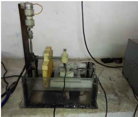
FIG 1: Showing the fabricated ECM setup
