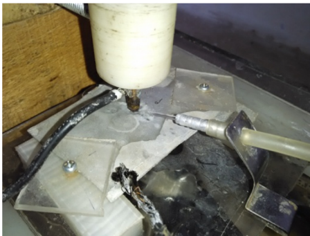
FIG 2: Showing the machining of Aluminium using Copper tool.
