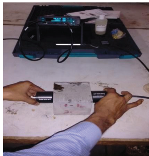
Figure 1. 'PUNDIT' Ultrasonic Pulse Velocity Device
