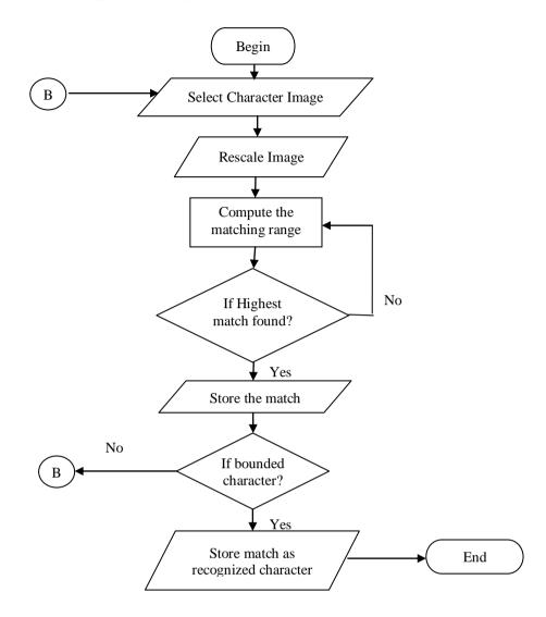
Figure 3. Flowchart for implementation of Template Matching for OCR
