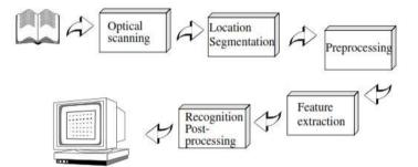
Figure 2. Components of OCR
