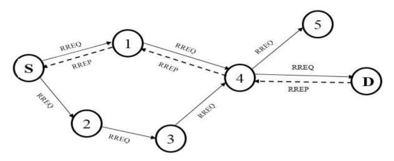
Figure 1. AODV Routing Protocol
