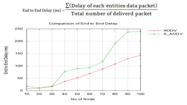
Figure 7. Compare End to End Delay of AODV with S\_AODV
