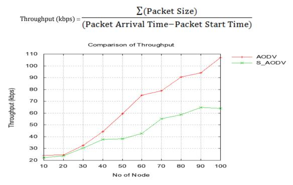
Figure 4. Compare Throughput of AODV with S\_AODV
