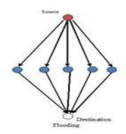
Figure-2.1 Flooding Protocol
