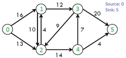
Figure 2. Ford Fulkerson Algorithm for Graph
