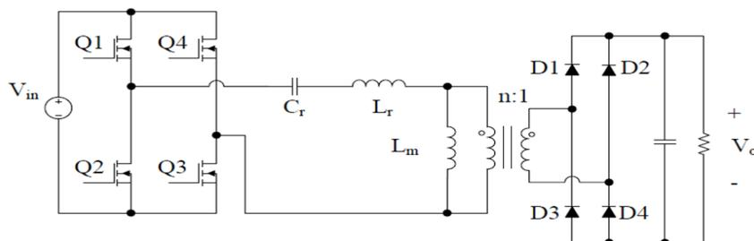
*Fig. 2: Full bridge LLC Resonant converter*
