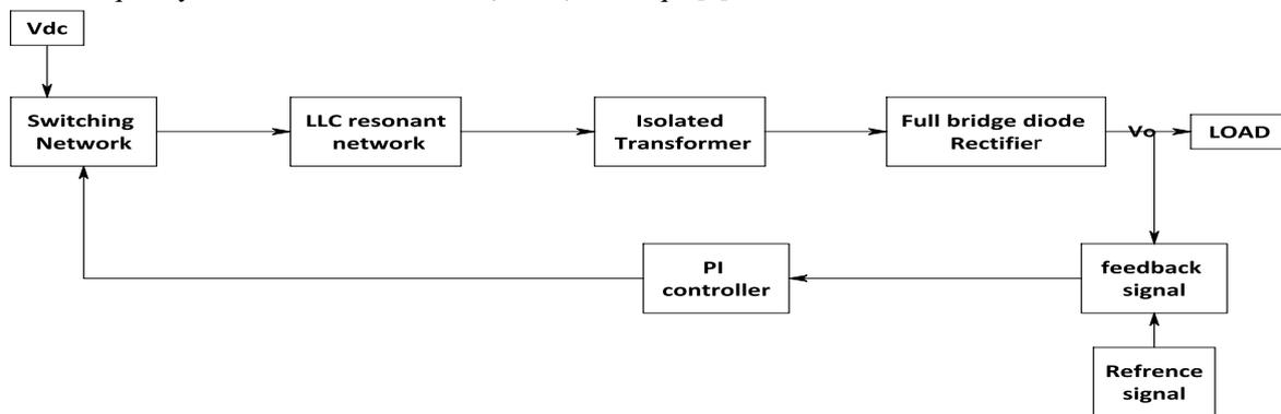
*Fig.1: block diagram of controlled LLC*
