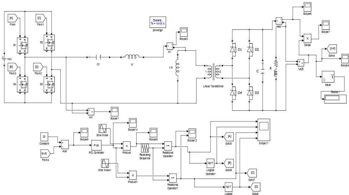
Fig.5: SPWM based close loop simulation
