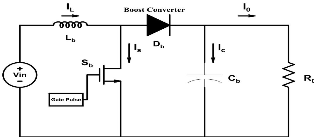
*Figure 1 Circuit diagram of a boost converter*
