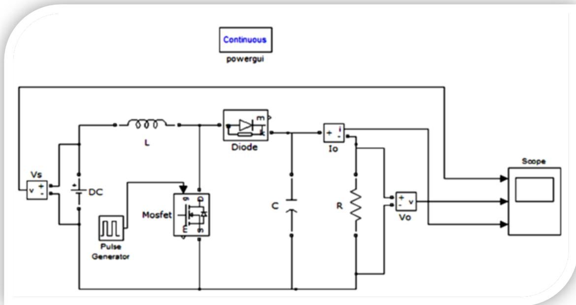
Figure 2 MATLAB model of open loop boost converter
