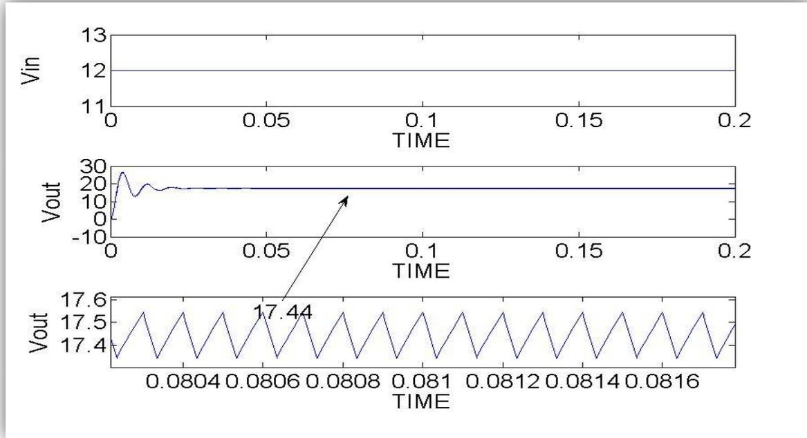
Figure 4 Waveforms open loop boost converter for input voltage of 12 V
