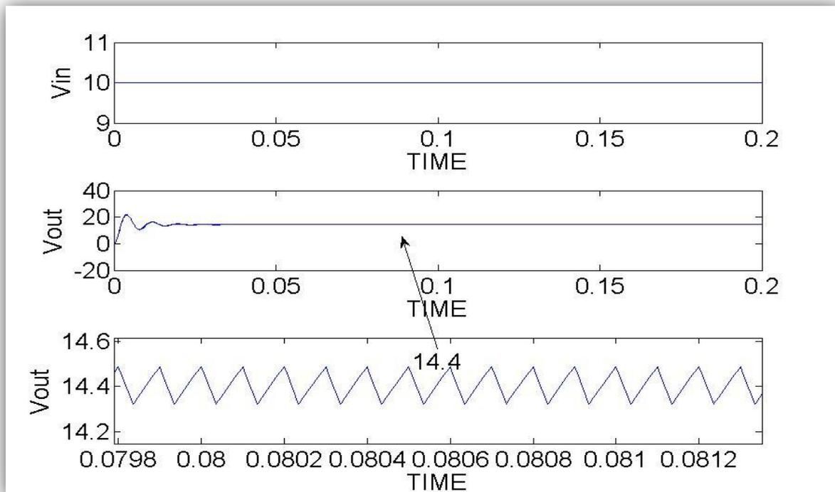
Figure 3 Waveforms open loop boost converter for input voltage of 10 V
