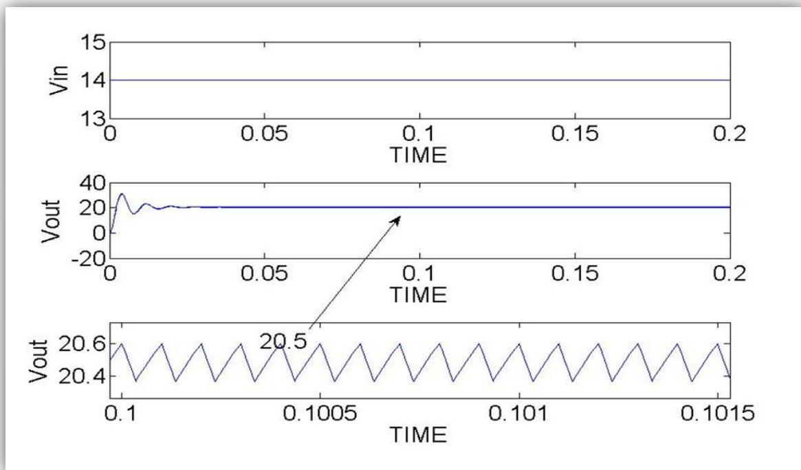
Figure 5 Waveforms open loop boost converter for input voltage of 14 V
