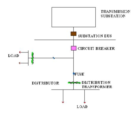
Figure 1: Radial Feeder Distribution System
