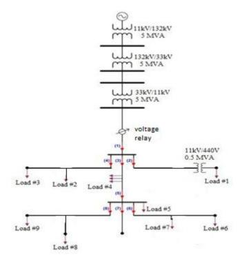
Fig. 2. Radial Feeder System-13 bus system
