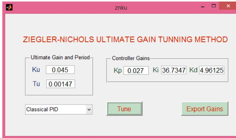
**Fig. 11 GUI application for ZN instability method**
