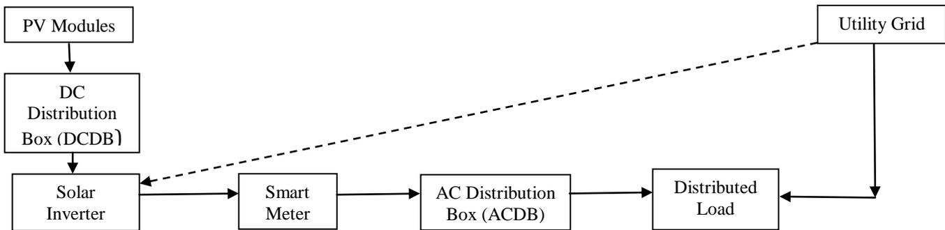
*Figure 1. Block diagram of PV plant*
