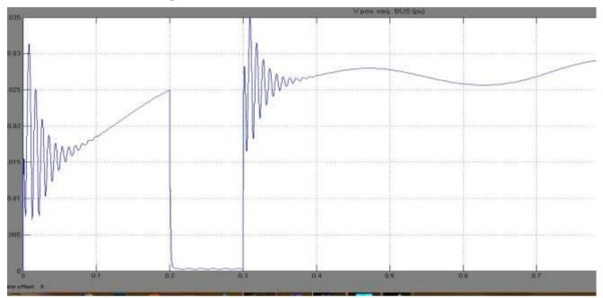
5.1.3.SMIB Waveform Of Voltage P.u V/S Time (LG Fault) with SVC
