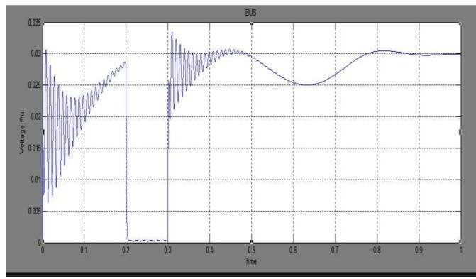
5.1.2.SMIB Waveform Of Voltage P.u V/S Time (LG Fault) without SVC
