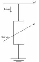
Fig.4. Equivalent Circuit Diagram of SVC [8]
