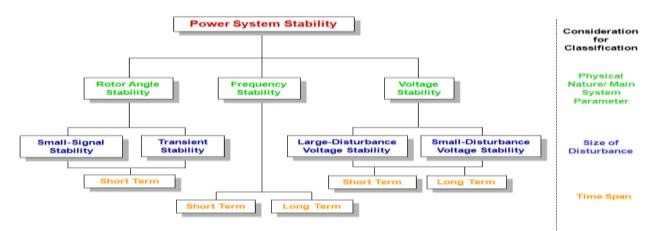
Fig.1 Classification of Power System Stability[1]
