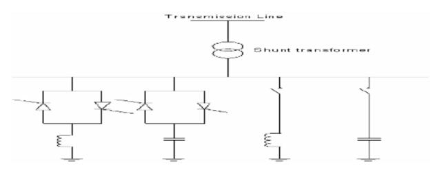
Fig.3. Single Line Diagram of SVC[18]
