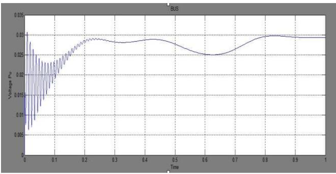
Fig.6.SMIB Waveform Of Voltage P.u V/S Time (During Normal Condition) without SVC
