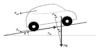
Figure 2.2 Forces on electric vehicle
