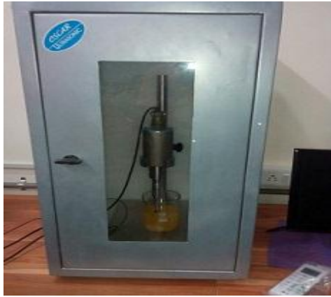
Fig. 2.3: Photograph of ultrasonic horn type processor
