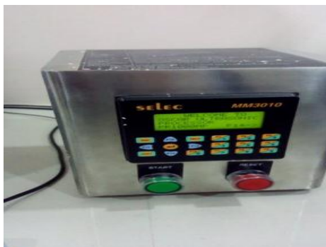
Fig. 2.4: Power unit of ultrasonic horn
