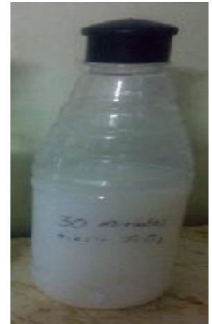
Fig.-3.6 T-0.25 nano fluid on 20 th day (30 minutes sonication)
