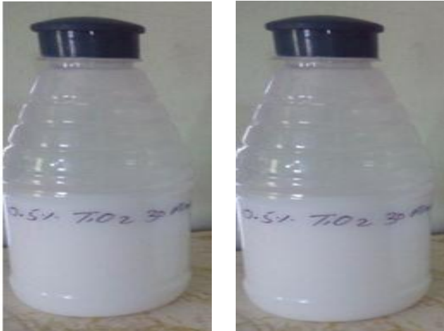
Fig.-3.9T-0.50 nano fluid on first day (30 minutes sonication) Fig.-3.10T-0.50 nano fluid on 18 th day (30 minutes sonication)
