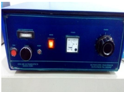
Fig. 2.4: Power unit of ultrasonic horn
