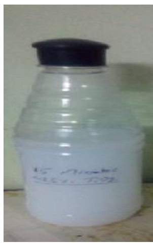
Fig.-3.4 T-0.25 nano fluid on 20 th day (15 minutes sonication)
