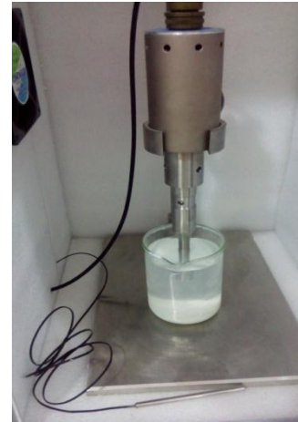
Fig 2.1:Preparation of nano fluid in ultra sonic horn machine
